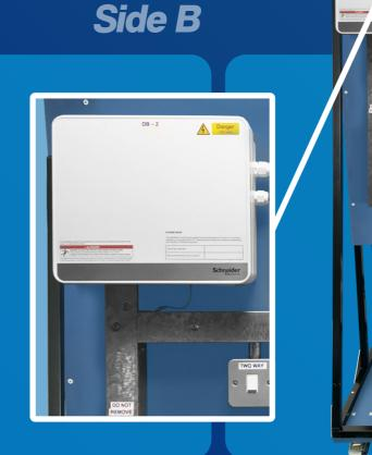
The rig incorporates single and 3 phase distribution areas with specific faults built into the circuits to prove competency in completing Minor Works, Electrical Installation Certificates and Electrical Installation Condition Reports. The 3 phase distribution board having SWA, MICC along with trunking & conduit wiring systems complete with main protective bonding simulation.
